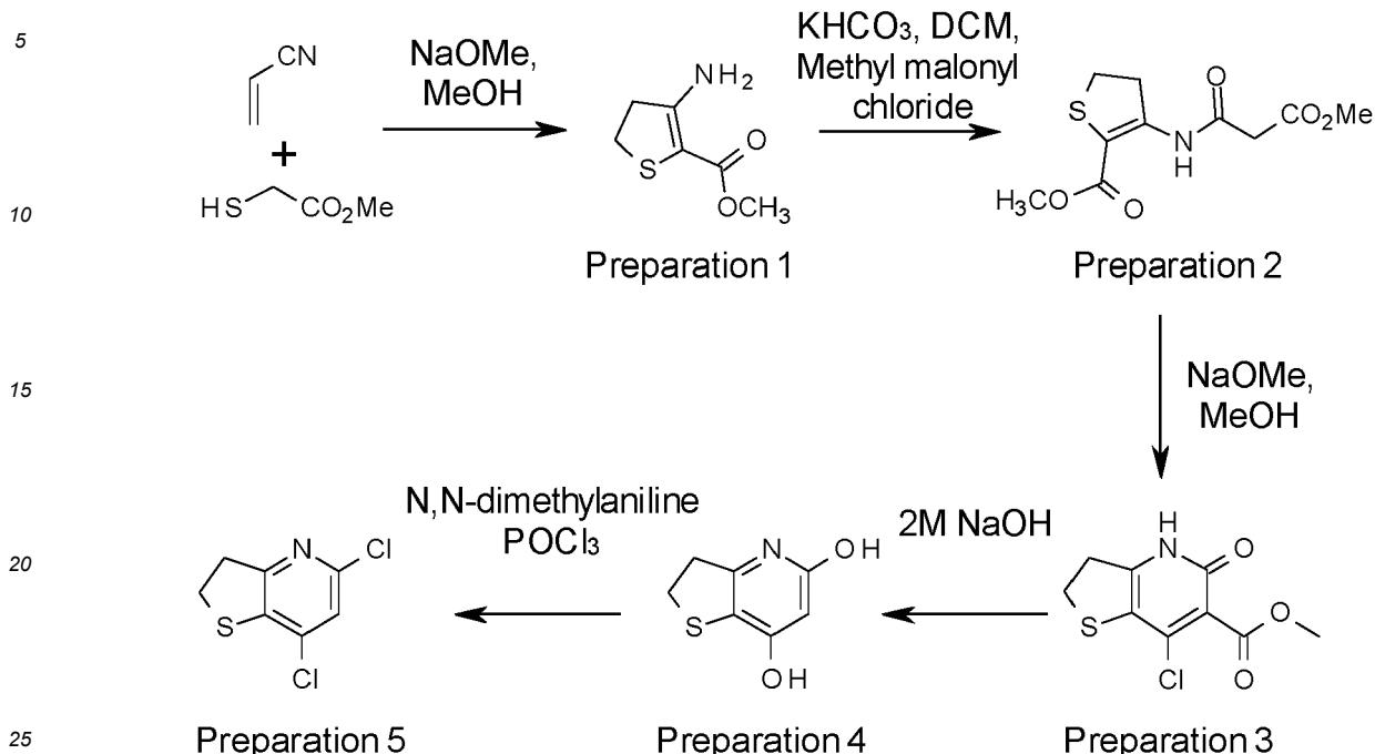
**[0098]** 5,7-Dichloro-2,3-dihydrothieno[3,2-b]pyridine can be prepared, as shown in Scheme 1, by the methods described in Preparations 1 to 5.
