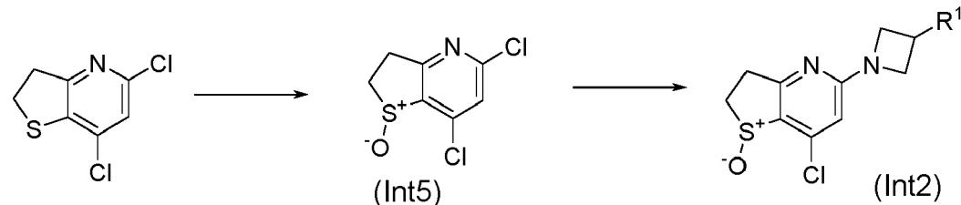
**[0105]** The sulfoxide of formula (Int5) can be prepared, as shown in Scheme 3, by reaction of 5,7-dichloro-2,3-dihydrothieno[3,2-b]pyridine (Preparation 5) with a suitable oxidising agent in an appropriate solvent, optionally in the presence of a chiral catalyst. For example, a solution of 5,7-dichloro-2,3-dihydrothieno[3,2-b]pyridine (Preparation 5) in EtOH/water can be oxidised by treatment with  $\text{NaIO}_4$ , at a temperature between 0°C and room temperature.
