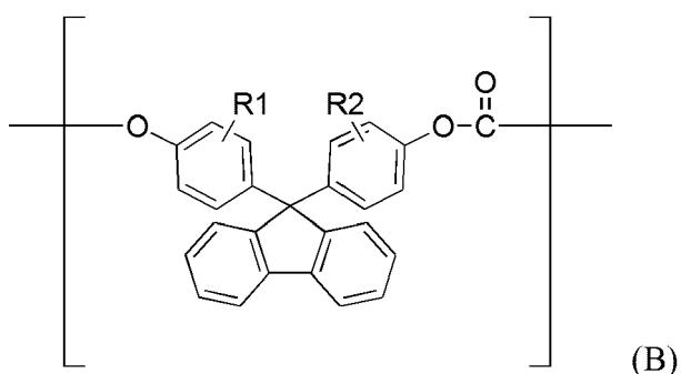
30 (in formula (B), R1 and R2 are each independently a hydrogen atom, an alkyl group having 1 to 20 carbon atoms, an alkoxy group having 1 to 20 carbon atoms, a cycloalkyl group having 5 to 20 carbon atoms, a cycloalkoxy group having 5 to 20 carbon atoms, an aryl group having 6 to 20 carbon atoms or an aryloxy group having 6 to 20 carbon atoms).
