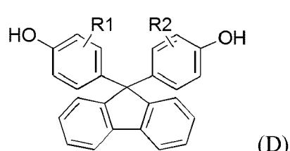
35 (in formula (D), R1 and R2 are each independently a hydrogen atom, an alkyl group having 1 to 20 carbon atoms, an alkoxyl group having 1 to 20 carbon atoms, a cycloalkyl group having 5 to 20 carbon atoms, a cycloalkoxyl group having 5 to 20 carbon atoms, an aryl group having 6 to 20 carbon atoms or an aryloxy group having 6 to 20 carbon atoms).
