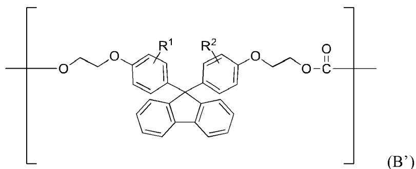
(in formula (B'), R1 and R2 are each independently a hydrogen atom, an alkyl group having 1 to 20 carbon atoms, an alkoxy group having 1 to 20 carbon atoms, a cycloalkyl group having 5 to 20 carbon atoms, a cycloalkoxyl group having 5 to 20 carbon atoms, an aryl group having 6 to 20 carbon atoms or an aryloxy group having 6 to 20 carbon atoms).
