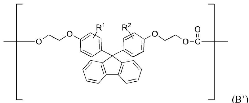
35 wherein, in formula (B'), R<sup>1</sup> and R<sup>2</sup> are each independently a hydrogen atom, an alkyl group having 1 to 20 carbon atoms, an alkoxy group having 1 to 20 carbon atoms, a cycloalkyl group having 5 to 20 carbon atoms, a cycloalkoxy group having 5 to 20 carbon atoms, an aryl group having 6 to 20 carbon atoms or an aryloxy group having 6 to 20 carbon atoms,
