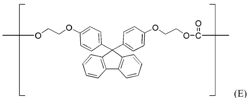
15 [0018] Moreover, Patent Document 10 discloses a polycarbonate resin comprising a structural unit having a fluorene structure and bisphenol A. In the Example section of this document, it is shown that this resin achieved a refractive index of 1.616 to 1.636. It should be noted that the structural unit disclosed in this document is distinct from formula (E).
