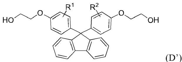
10 (in formula (D'), R<sup>1</sup> and R<sup>2</sup> are each independently a hydrogen atom, an alkyl group having 1 to 20 carbon atoms, an alkoxy group having 1 to 20 carbon atoms, a cycloalkyl group having 5 to 20 carbon atoms, a cycloalkoxyl group having 5 to 20 carbon atoms, an aryl group having 6 to 20 carbon atoms or an aryloxy group having 6 to 20 carbon atoms).
