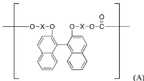
wherein, in formula (A), X is an alkylene group having 1 to 4 carbon atoms, wherein the resin has an orientation birefringence  $\Delta n$  of  $1.0 \times 10^{-3}$  or less, and wherein the orientation birefringence  $\Delta n$  is determined by calculation according to the following equation:
