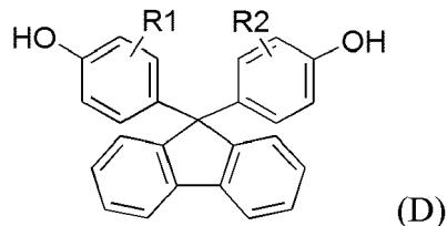
15 wherein, in formula (D), R<sup>1</sup> and R<sup>2</sup> are each independently a hydrogen atom, an alkyl group having 1 to 20 carbon atoms, an alkoxy group having 1 to 20 carbon atoms, a cycloalkyl group having 5 to 20 carbon atoms, a cycloalkoxy group having 5 to 20 carbon atoms, an aryl group having 6 to 20 carbon atoms or an aryloxy group having 6 to 20 carbon atoms.
