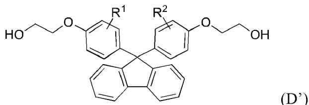
25 (in formula (D'), R<sup>1</sup> and R<sup>2</sup> are each independently a hydrogen atom, an alkyl group having 1 to 20 carbon atoms, an alkoxy group having 1 to 20 carbon atoms, a cycloalkyl group having 5 to 20 carbon atoms, a cycloalkoxyl group having 5 to 20 carbon atoms, an aryl group having 6 to 20 carbon atoms or an aryloxy group having 6 to 20 carbon atoms).
