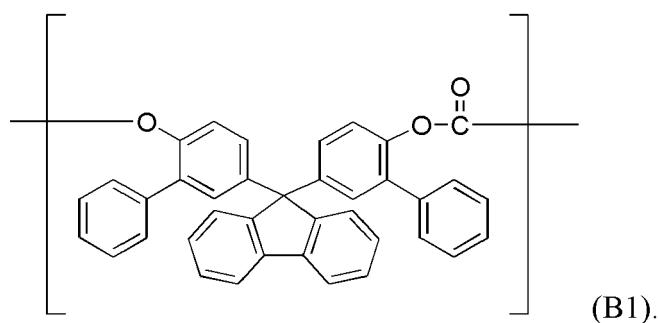
20. The polycarbonate resin according to any one of claims 12 to 19, wherein the structural unit (B2) is a structural unit (B2) represented by the following formula:
