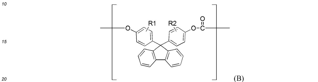
(in formula (B), R1 and R2 are each independently a hydrogen atom, an alkyl group having 1 to 20 carbon atoms, an alkoxy group having 1 to 20 carbon atoms, a cycloalkyl group having 5 to 20 carbon atoms, a cycloalkoxy group having 5 to 20 carbon atoms, an aryl group having 6 to 20 carbon atoms or an aryloxy group having 6 to 20 carbon atoms).
