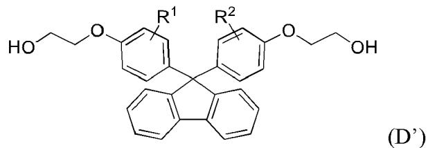
35     wherein, in formula (D'), R<sup>1</sup> and R<sup>2</sup> are each independently a hydrogen atom, an alkyl group having 1 to 20 carbon atoms, an alkoxy group having 1 to 20 carbon atoms, a cycloalkyl group having 5 to 20 carbon atoms, a cycloalkoxy group having 5 to 20 carbon atoms, an aryl group having 6 to 20 carbon atoms or an aryloxy group having 6 to 20 carbon atoms.
