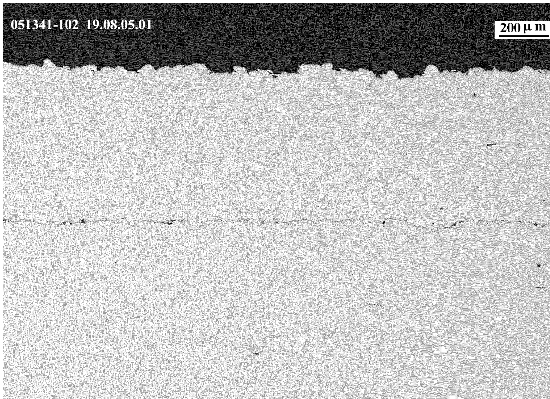
FIG. 11 Tool steel (Heatvar) as sprayed metallographic cross section
