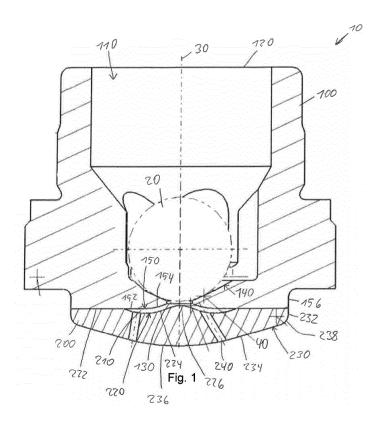
**[0001]** The invention relates to a valve seat body assembly for a fluid injector of an internal combustion engine, wherein the valve seat body assembly comprises a valve seat body which extends in axial and radial direction with respect to a central longitudinal axis and an orifice part which is arranged at the valve seat body.
