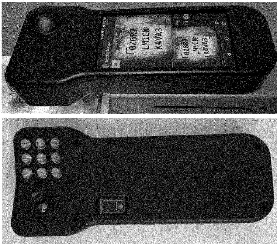
Figure 7: Upper and lower shell of the LWIR imaging system in the form of a handheld housing
