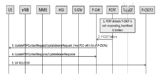
Fig. 3: P-CSCF Failure Detection by PCRF
