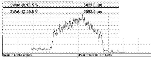
Laser Output Beam Profile – Flow Axis
