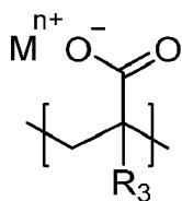
10 wherein R<sub>2</sub> and R<sub>3</sub> are independently of each other hydrogen or a C1 to C6 alkyl group, M<sup>n+</sup> is a cation having an oxidation number of n, and n is an integer of 1 to 3,
