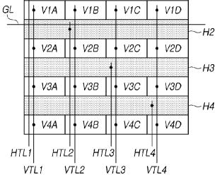
► Horizontal Direction V1 = V1A + V2A + V3A + V4AV2 = V1B + V2B + V3B + V4BV3 = V1C + V2C + V3C + V4CVertical Direction V4 = V1D + V2D + V3D + V4D
