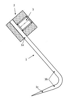
**[0001]** The subject of the invention is a needle gripper (Fig. 1) for gripping various workpieces by means of physical perforation of the workpiece executed by a curved sharp tip of the gripping needle, where the straight part
