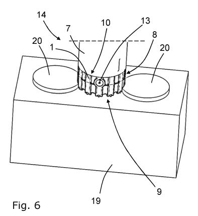
[0001] The current invention relates to a tool comprising a base element and studs that are provided on the base element. The invention further relates to a method for forming such a tool and to a use of such a tool for forming secant walls.
