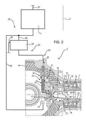
[0001] The present invention relates to a transmission assembly for an aircraft capable of hovering.
