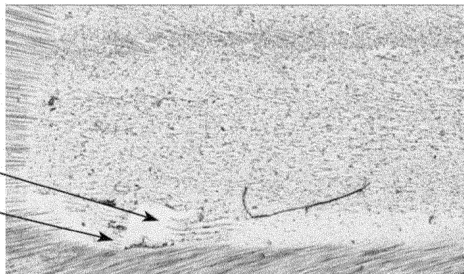
(c) TOOTH FLANK FAILURE INITIATION STATE OF HELICAL GEAR FOR PASSENGER CAR (MESHING START POINT OF TOOTH OF DRIVING GEAR)
