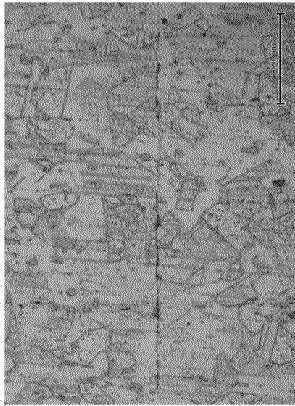
Example 28 AMPCO940 (Cu-2.3Ni-0.6Si-0.5Cr) Bonding surface obviously remains.
