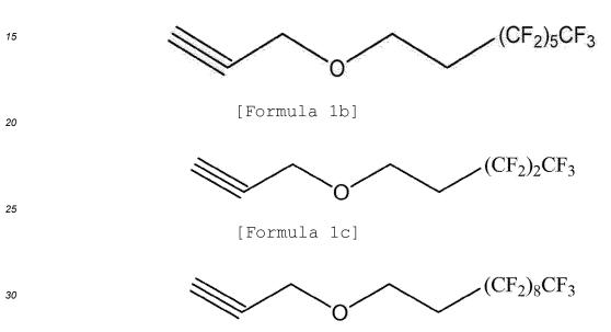
**[0046]** Meanwhile, the compound represented by Formula 1 may be included in an amount of 0.01 wt% to 10.0 wt% based on the total weight of the non-aqueous electrolyte solution for a lithium secondary battery.
