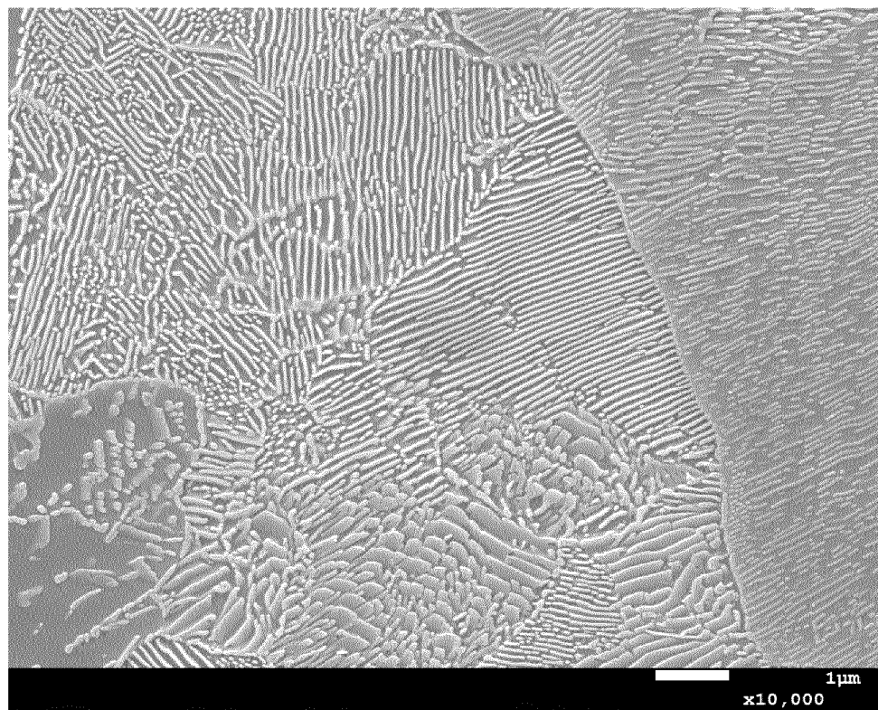
SWRH62A, CONVENTIONAL PRODUCT-LEAD FURNACE TEMPERATURE 565°C: SEM IMAGE
