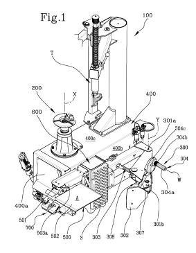
[0001] This invention relates to a tyre changing machine and to a method for using a tyre changing machine. [0002] The invention applies in particular to the automotive field and, more specifically, to the sector of vehicle service equipment and tyre changers.
