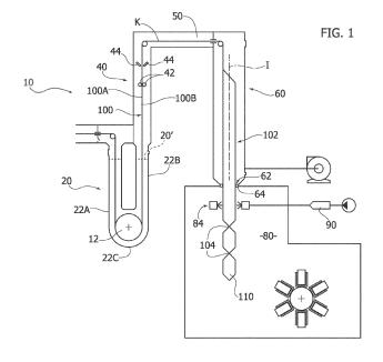
**[0001]** The present invention regards a method for producing containers filled with a product and sealed starting from a web of packaging material, the method comprising the steps of:
