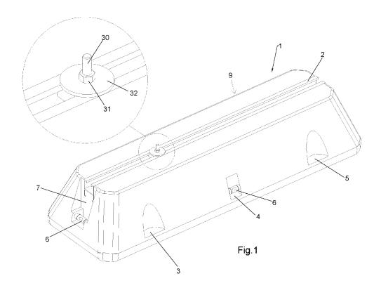
[0001] The present invention concerns an anti-vibration mount for the external units of air-conditioning equipment, wherein said air-conditioning equipment is placed outside buildings and generally rested on flat surfaces.
