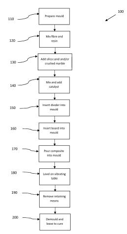
**[0001]** The present invention relates to a method of manufacturing a prefabricated insulated panel or sill.
