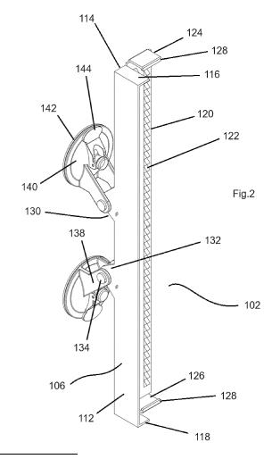
[0001] The present invention relates to apparatus for mounting a display board to a support surface and in particular, but not exclusively, to apparatus for mounting an advertising board to a window of a building.
