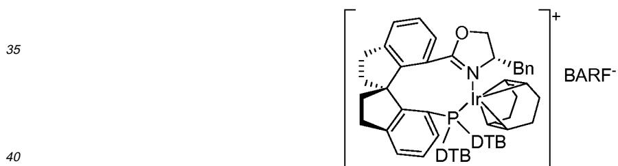
45 is used, the asymmetric catalytic hydrogenation of 2 - phenylethyl acrylic acid **9** is carried out under the condition same to that of Embodiment 6, the result of the reaction is that: the conversion rate is 100%, the yield is 91 % and the ee value of the product is 36%.
