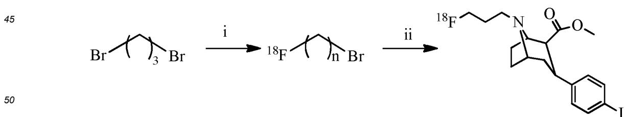
55 [0045] This method can be readily converted to be a method of the present invention by carrying out step (ii) in an aqueous alkanol solution using an aliquot of  $\text{K}_2\text{CO}_3$  and Kryptofix 222 (with acetonitrile removed) used to make reactive  $[^{18}\text{F}][\text{K}(\text{Kryptofix})]\text{F}$  for use in step (i).
