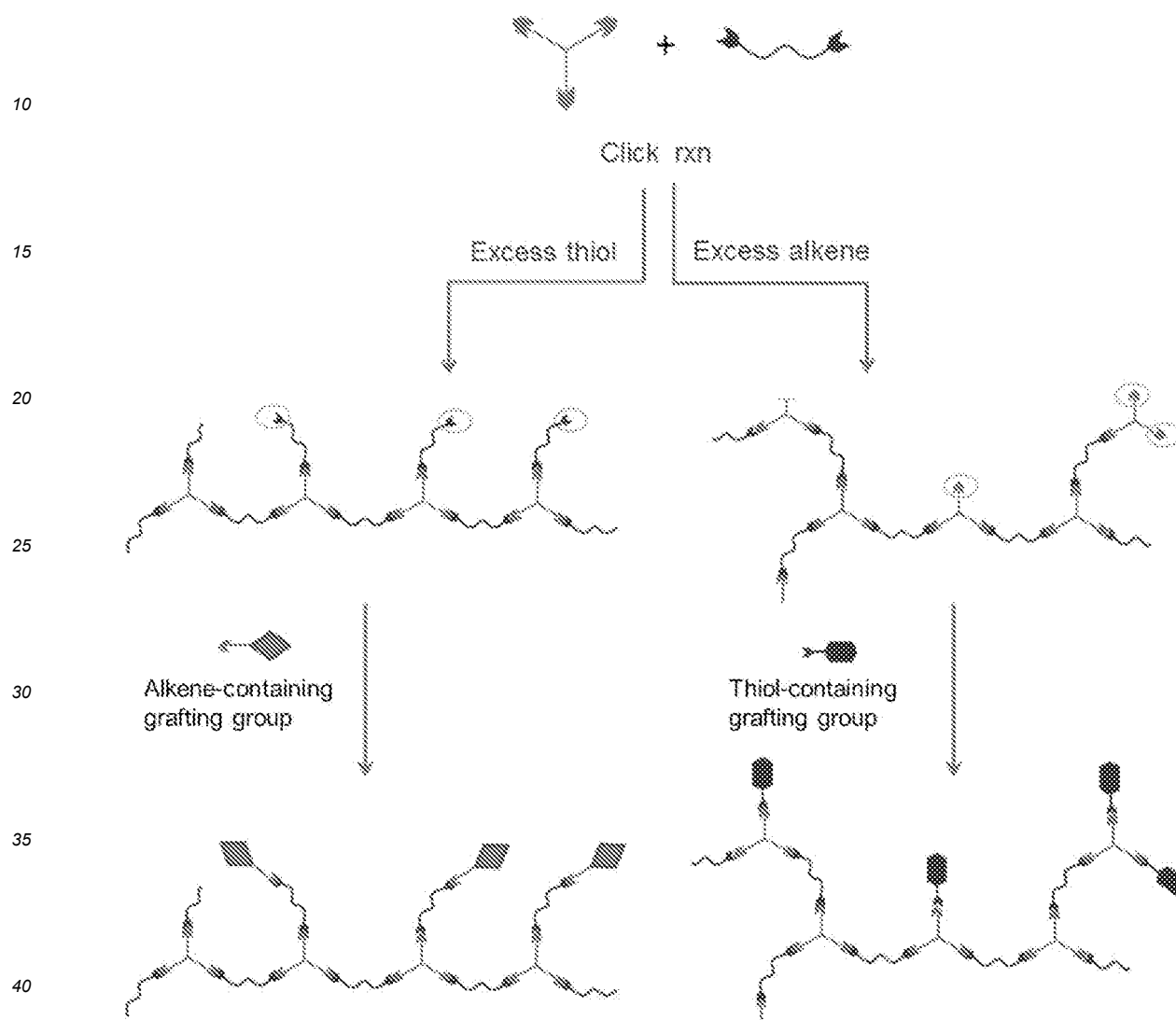
Scheme 3 – Two-step production method to produce grafted thiol-ene click polymers
